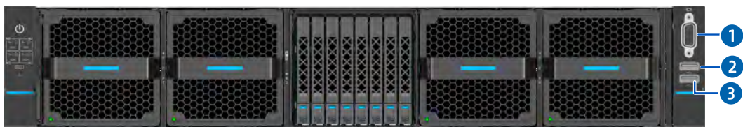
Figure 5-7 Front Panel Port Locations
