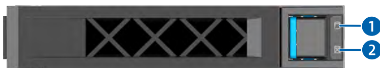
Figure 5-21 NVMe Drive LEDs
