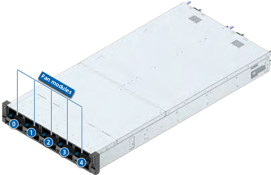
Figure 5-27 Front Fan Module Locations
