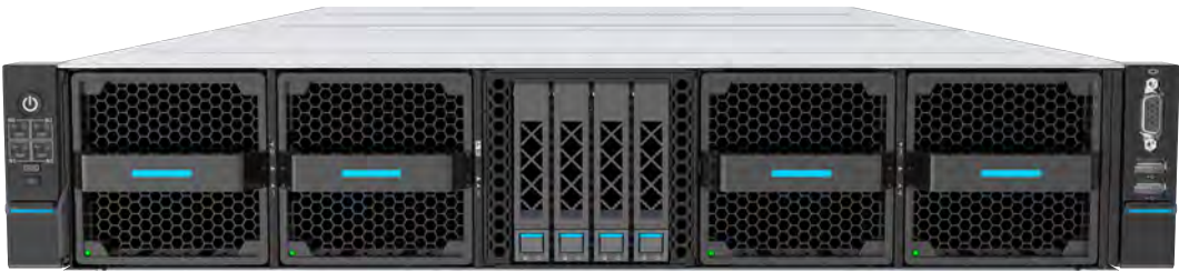
Figure 1-5 K24-X2-C0-R0-00 (4 × 2.5-inch Drive + 2 × 8080 Fan Configuration)
