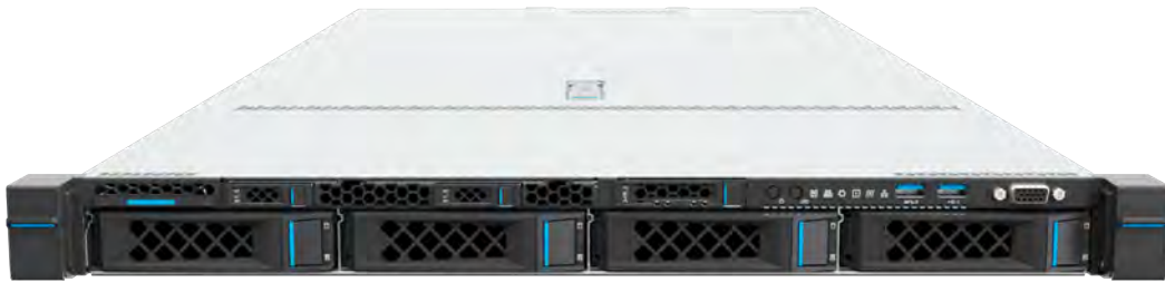
Figure 1-1 Appearance (4 × 3.5-Inch Drive + 2 × E1.S SSD + 2 × M.2 SSD Configuration)
