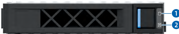
Figure 5-14 SAS/SATA Drive LEDs
