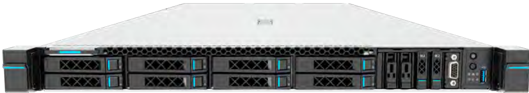
Figure 1-5 8 × 2.5-Inch Drive + 2 × E1.S SSD + 2 × M.2 SSD Configuration
