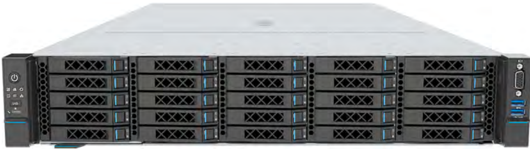
Figure 1-3 25 × 2.5-Inch Drive Configuration
