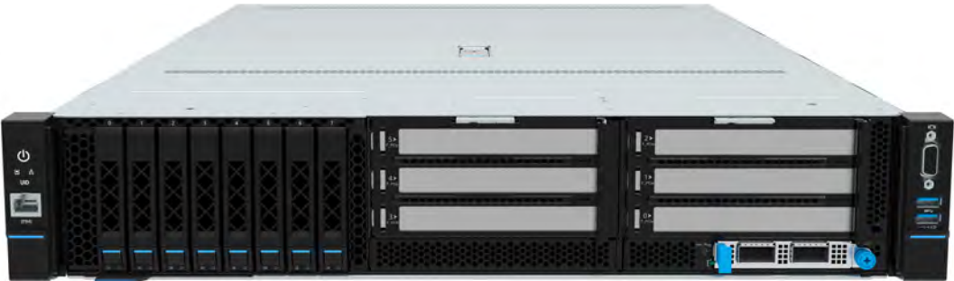
Figure 1-5 8 × 2.5-Inch Drive Configuration
