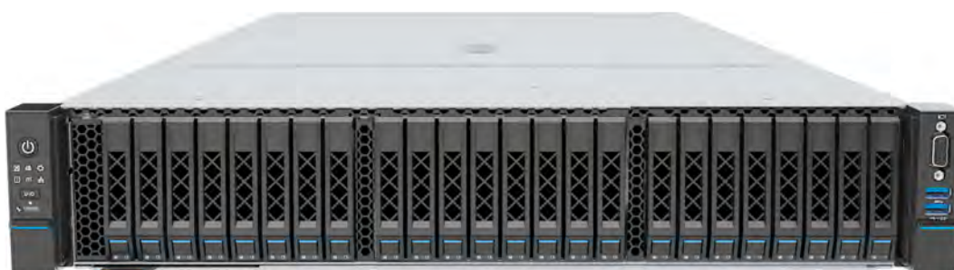
Figure 1-2 24 × 2.5-Inch Drive Configuration
