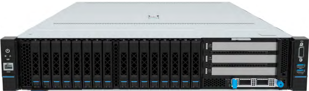
Figure 1-6 16 × 2.5-Inch Drive Configuration
