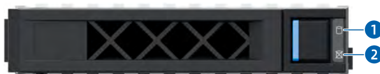
Figure 5-23 SAS/SATA Drive LEDs
