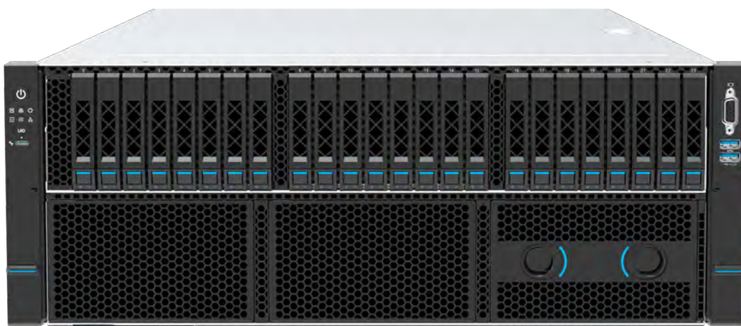
Figure 1-1 24 × 2.5-Inch Drive Configuration
