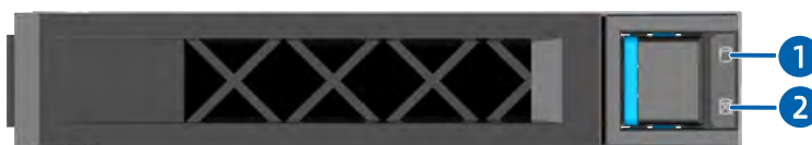
Figure 5-21 SAS/SATA Drive LEDs
