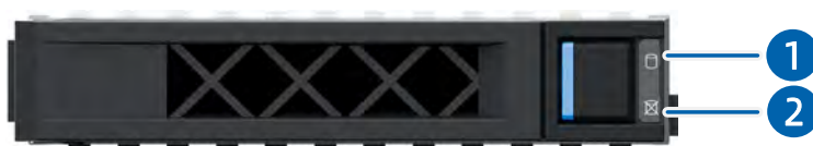
Figure 5-11 SAS/SATA Drive LEDs
