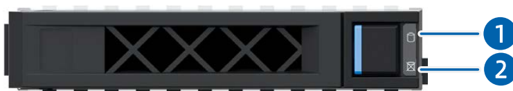
Figure 5-11 SAS/SATA Drive LEDs
