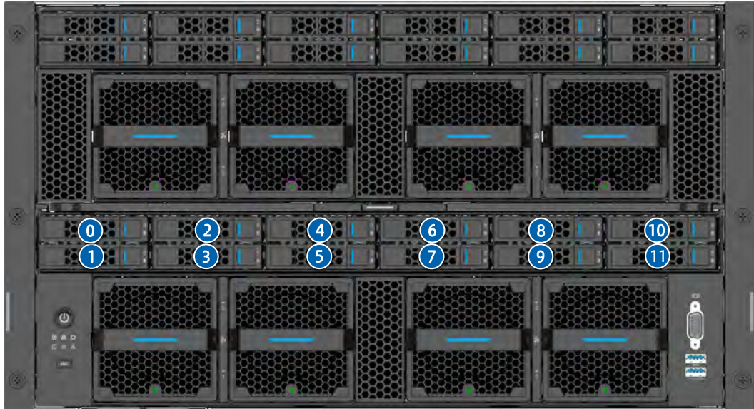
Figure 5-7 Drive Numbering (with an 8i RAID Card)
