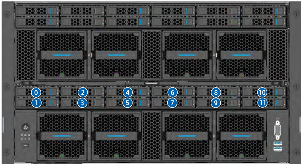
Figure 5-8 Drive Numbering (with a 16i RAID Card)
