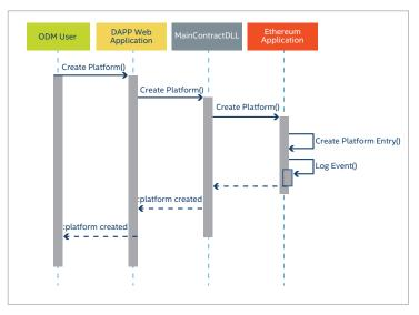
Figure 2. Platform Creation Sequence Diagram
